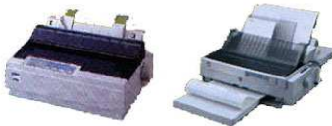
Gambar 1.11 Printer Dot Matrix 9 pin dan 24 pin
